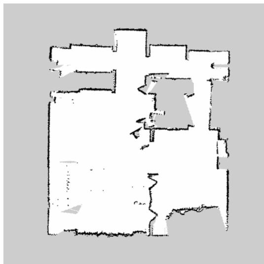
Figure 2: Map generated using grid map based SLAM
